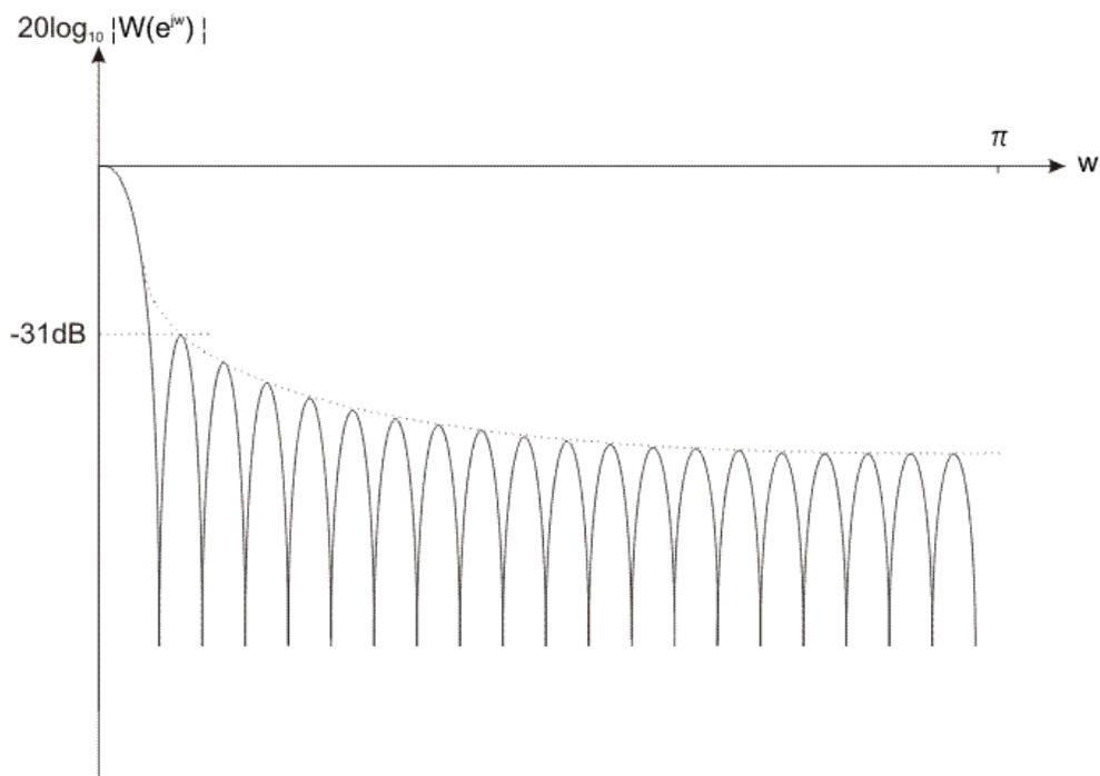
Figure 2-3-7. The Hann window coefficients in the frequency domain
