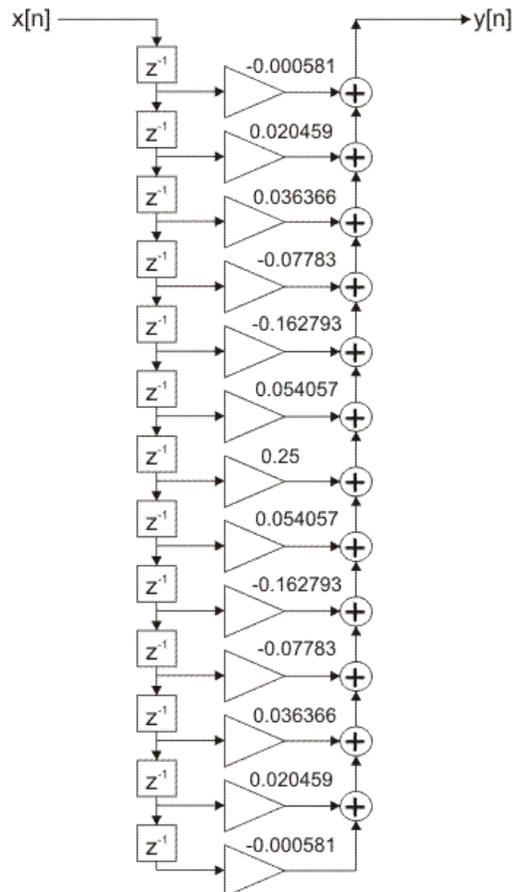
Figure 2-4-21. FIR filter direct realization
