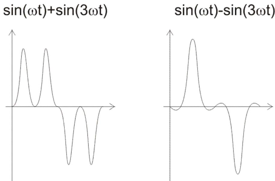
Figure 2-1-3. The effect of non-linear phase characteristic
