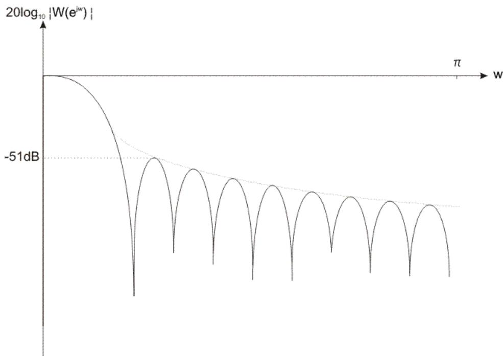
Figure 2-3-15. The Blackman window coefficients in the frequency domain
