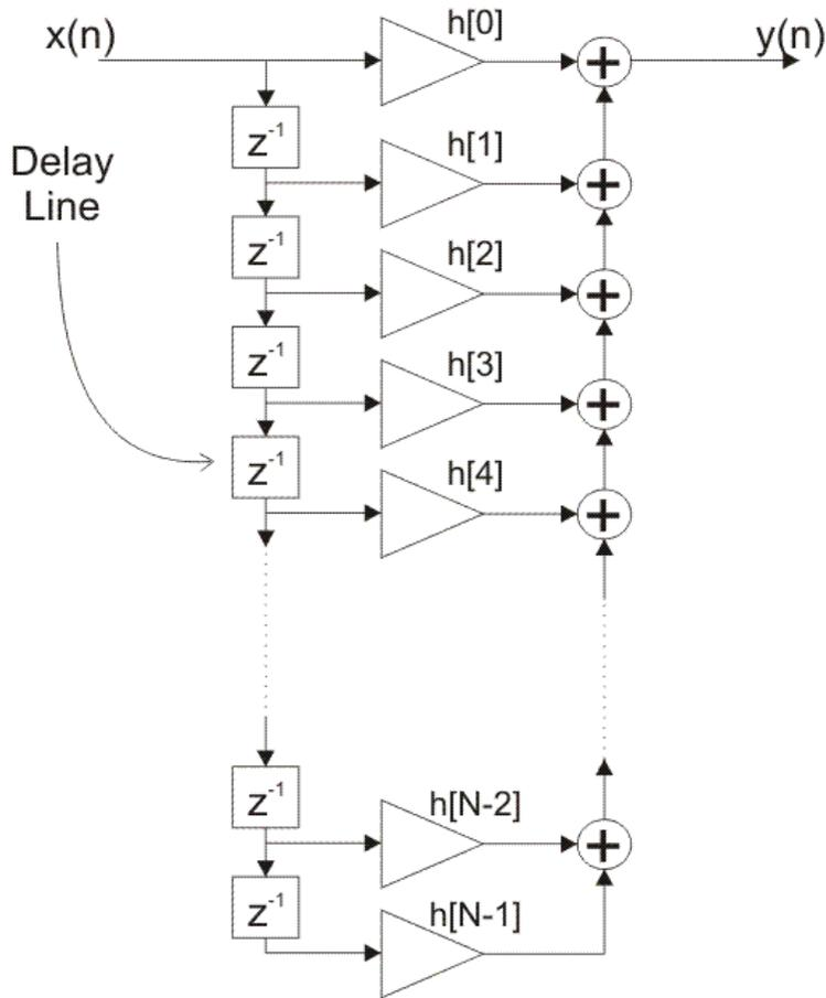
Figure 2-2-11. FIR filter direct realization
