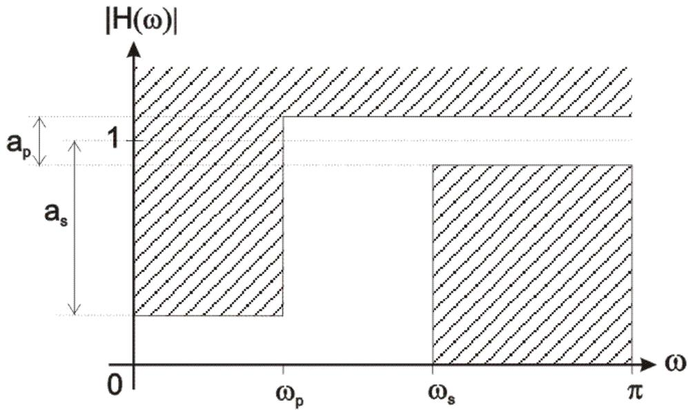
Figure 2-2-2b. High-pass digital filter specification
