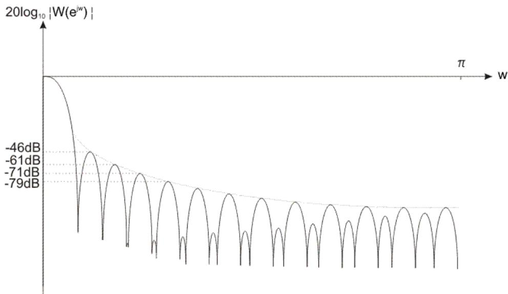
Figure 2-3-13. The Bohman window coefficients in the frequency domain
