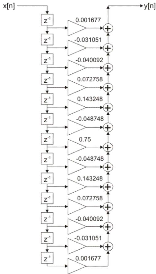
Figure 2-4-15. FIR filter direct realization
