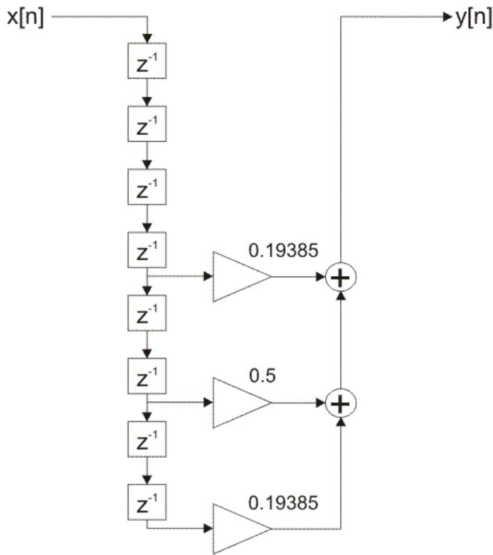
Figure 2-4-52. FIR filter direct realization
