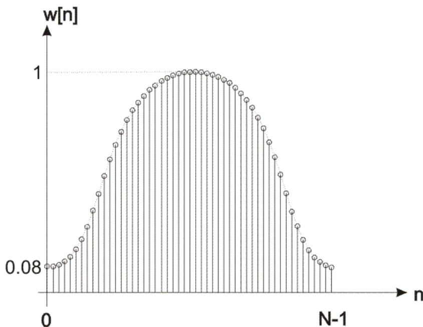
Figure 2-3-10. The Hamming window coefficients in the time domain
