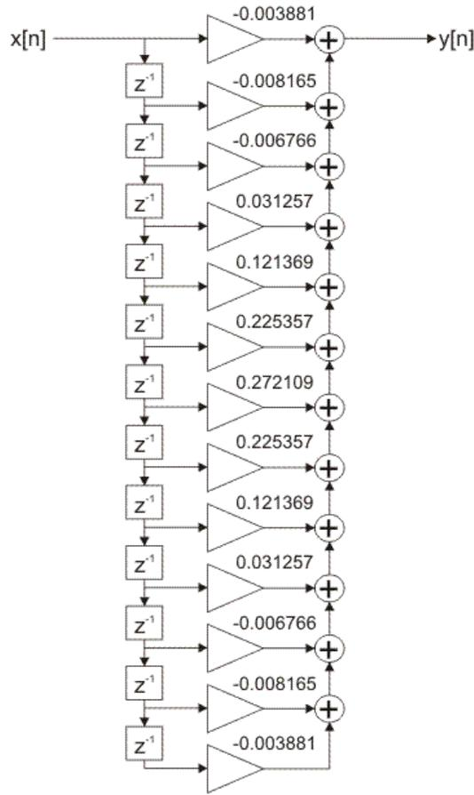
Figure 2-4-35. FIR filter direct realization
