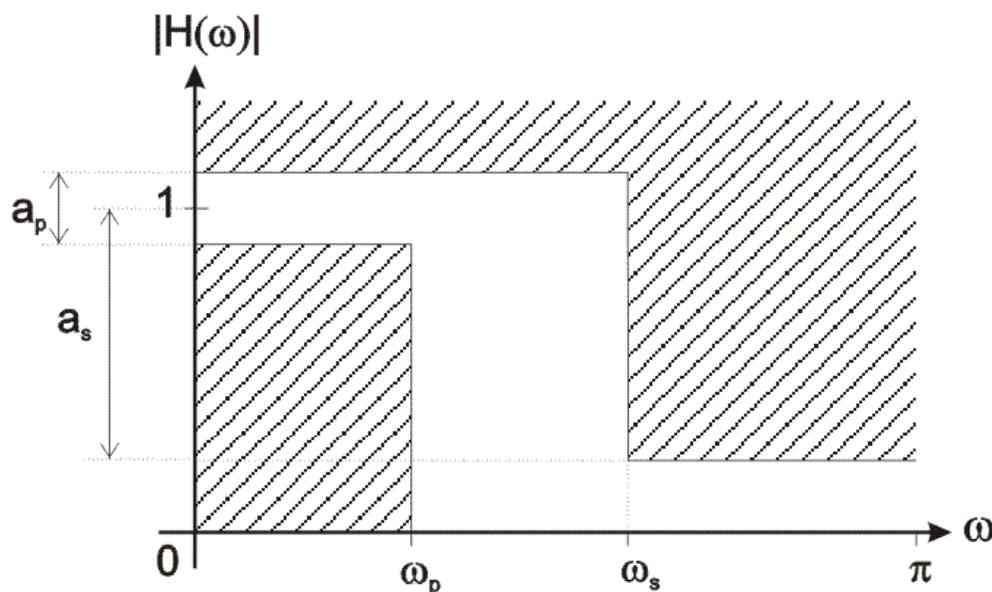
Figure2-2-1b. Low-pass digital filter specification
