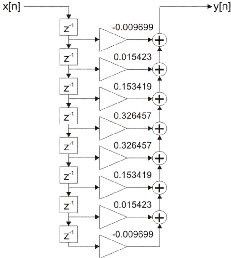
Figure 2-4-25. FIR filter direct realization
