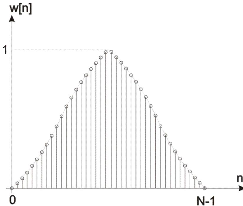
Figure 2-3-8. The Bartlett-Hanning window coefficients in the time domain
