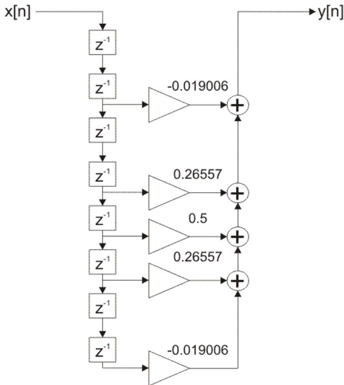
Figure 2-4-43. FIR filter direct realization
