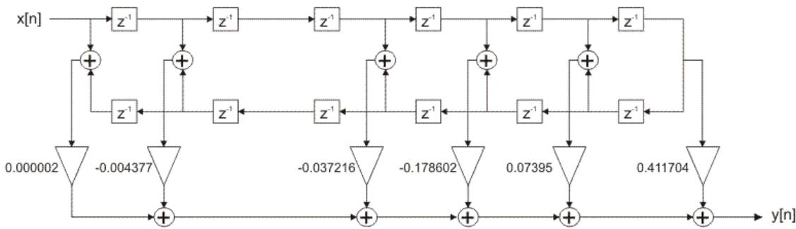
Figure 2-4-67. Optimized FIR filter design
