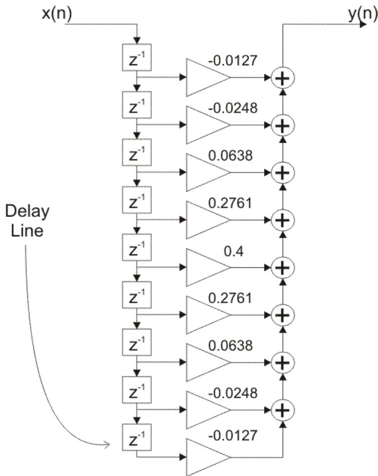
Figure 2-2-8. FIR filter realization
