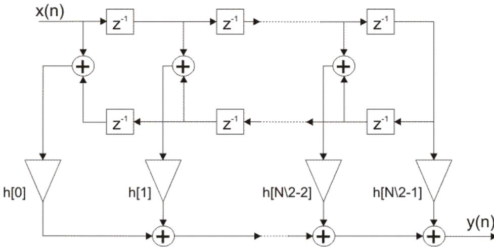
Figure 2-2-15. Optimized realization for odd frequency response
