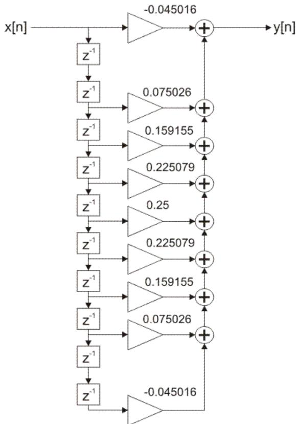
Figure 2-4-1. FIR filter direct realization
