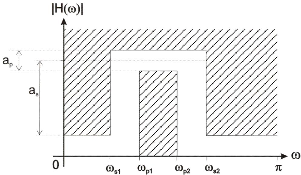
Figure 2-2-3b. Band-pass digital filter specification
