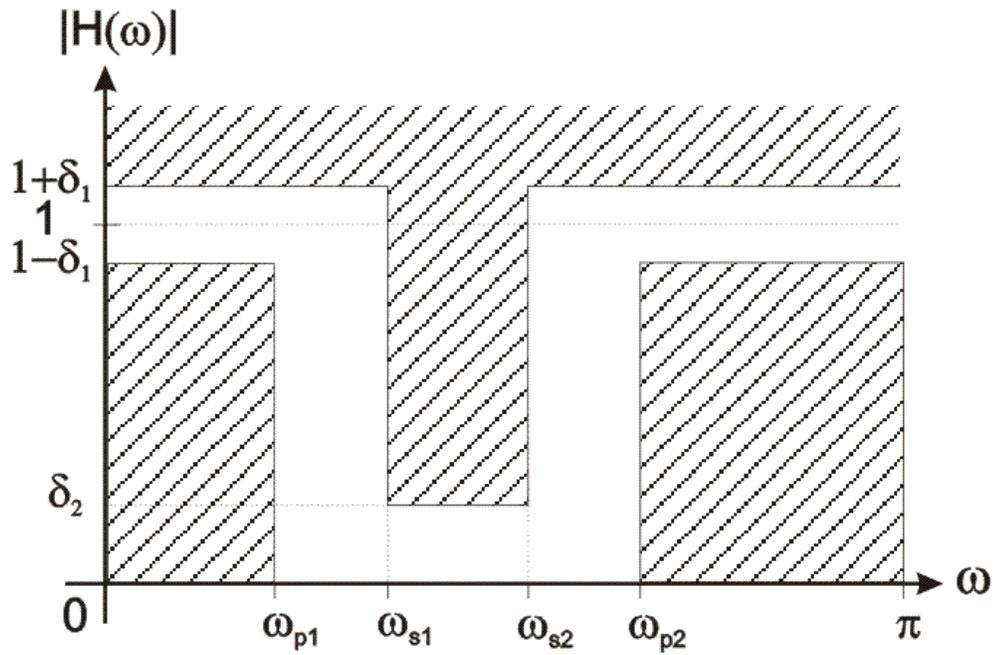
Figure 2-2-4a. Band-stop digital filter specification
