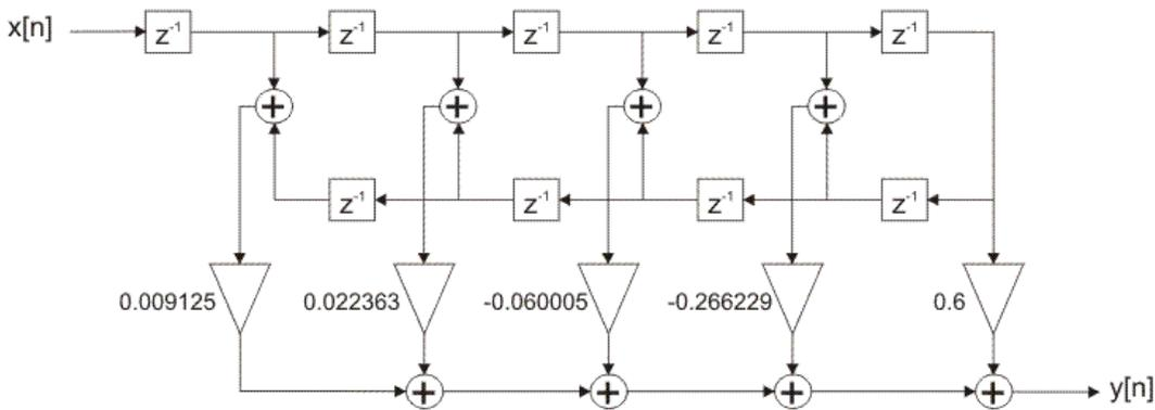
Figure 2-4-28. FIR filter optimized realization structure
