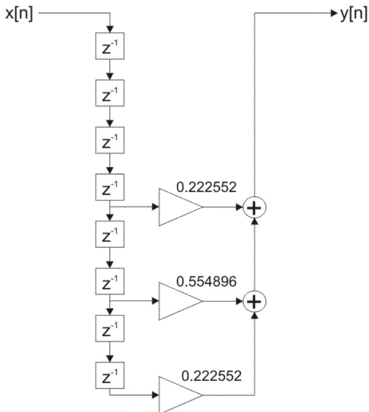
Figure 2-4-60. FIR filter direct realization
