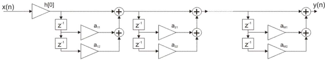
Figure 2-2-14. FIR filter cascade realization
