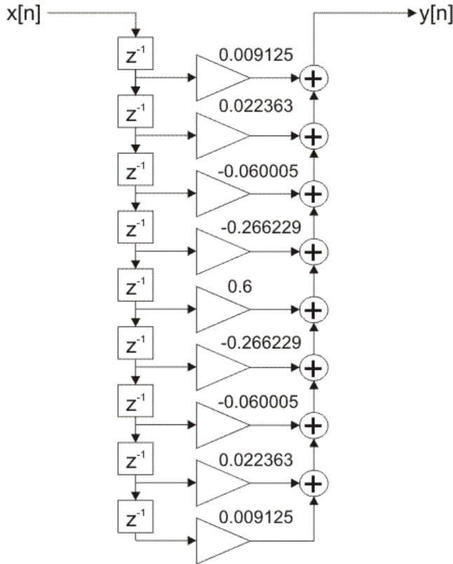
Figure 2-4-27. FIR filter direct realization
