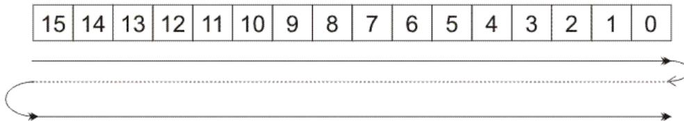
Figure 2-2-12. Circular buffer of length  $16 = 2^4$
