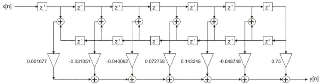
Figure 2-4-16. FIR filter optimized realization structure
