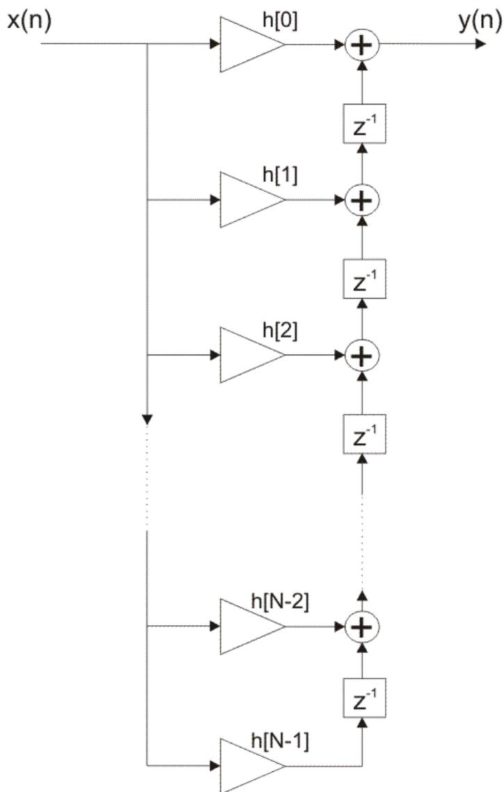
Figure 2-2-13. Direct transpose realization of a FIR filter
