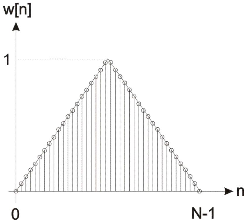
Figure 2-3-4. Triangular window coefficients in the time-domain
