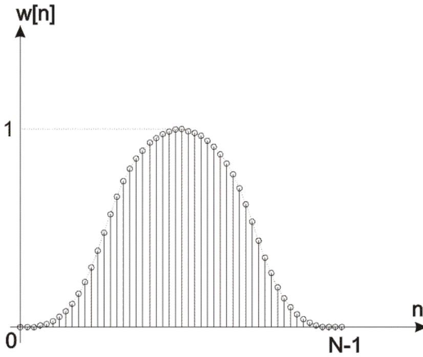
Figure 2-3-12. The Bohman window coefficients in the time domain
