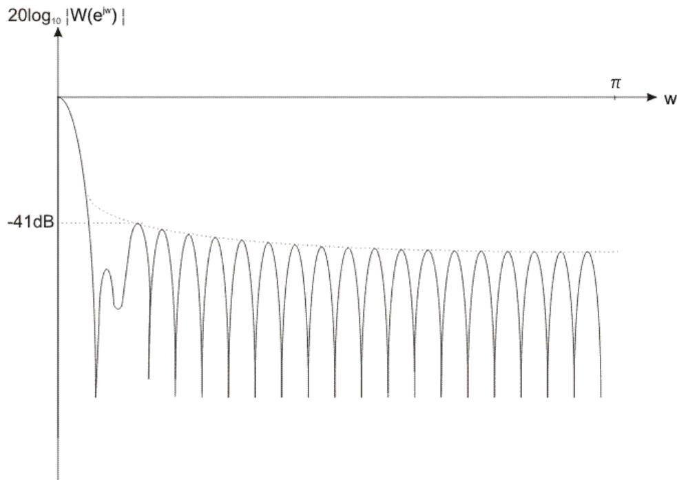
Figure 2-3-11. The Hamming window coefficients in the frequency domain
