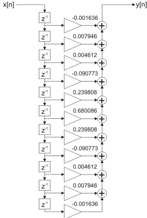
Figure 2-4-54. FIR filter direct realization
