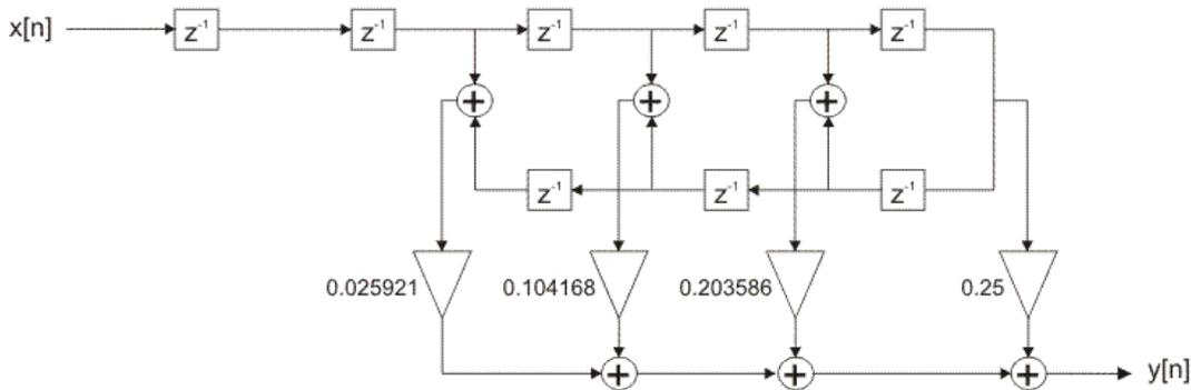
Figure 2-4-18. FIR filter optimized realization structure
