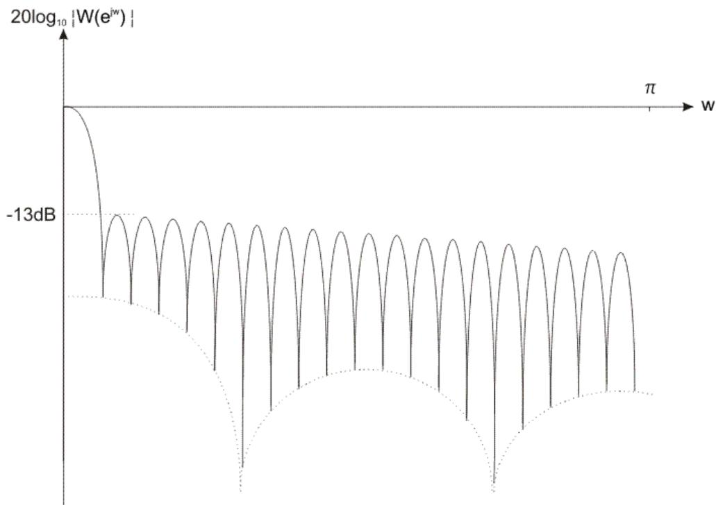
Figure 2-3-3. Rectangular window in the frequency domain (spectrum)
