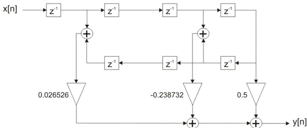
Figure 2-4-12. FIR filter optimized realization structure
