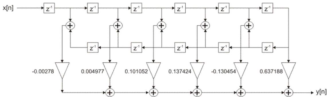
Figure 2-4-32. FIR filter optimized realization structure
