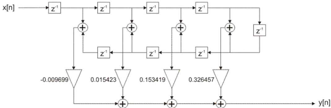
Figure 2-4-26. FIR filter optimized realization structure
