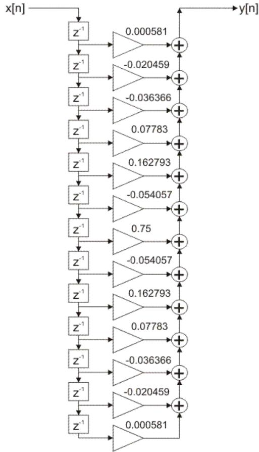
Figure 2-4-23. FIR filter direct realization
