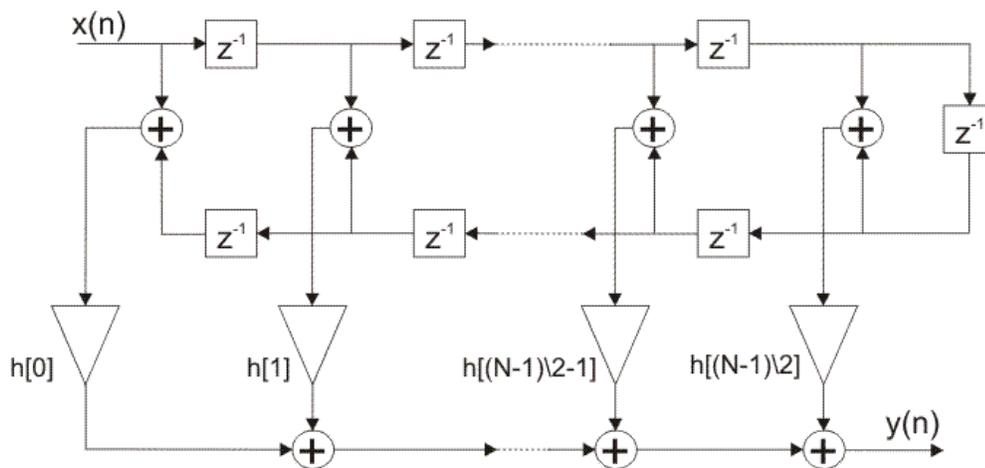
Figure 2-2-16. Optimized realization for even frequency response
