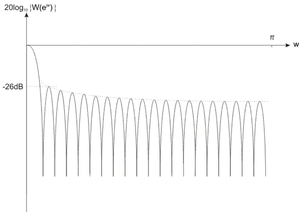
Figure 2-3-5. Triangular (Bartlett) window in the frequency domain (spectrum)
