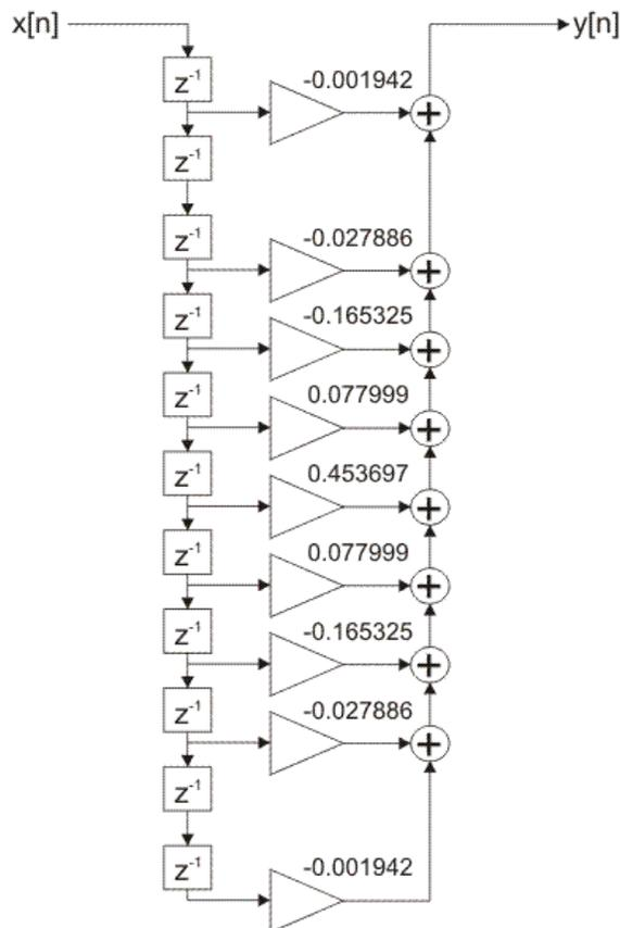
Figure 2-4-58. FIR filter direct realization
