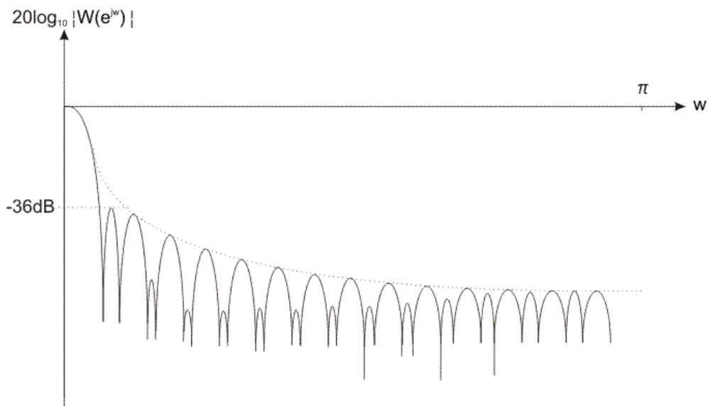
Figure 2-3-9. The Bartlett-Hanning window coefficients in the frequency domain
