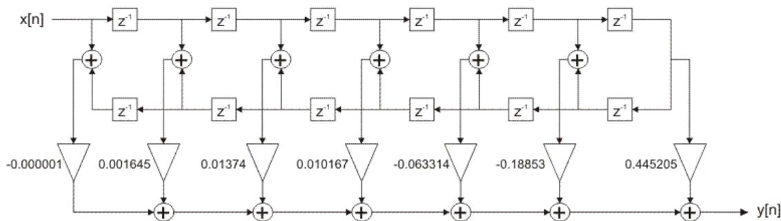
Figure 2-4-65. Optimized FIR filter design
