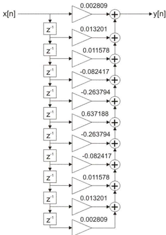
Figure 2-4-37. FIR filter direct realization
