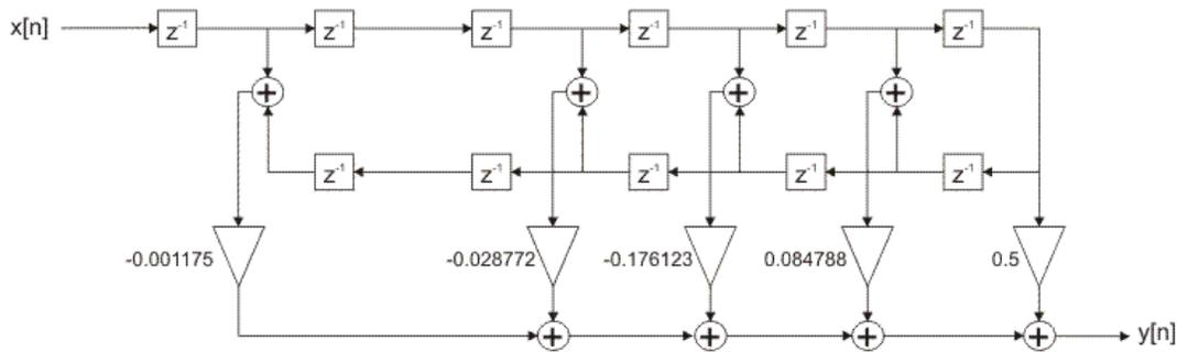
Figure 2-4-51. FIR filter optimized realization structure
