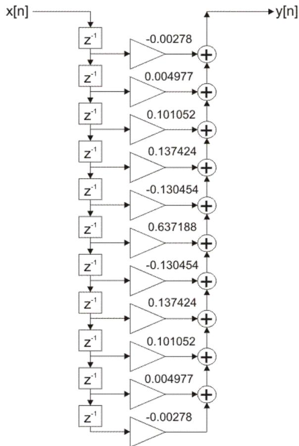
Figure 2-4-31. FIR filter direct realization
