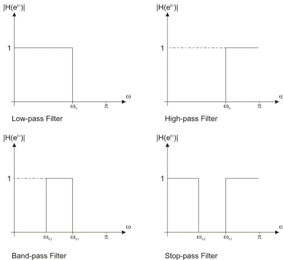
Figure 2-2-10. Transfer functions of four standard ideal filters
