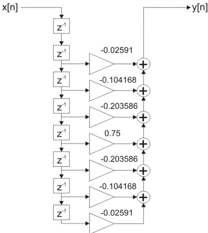
Figure 2-4-19. FIR filter direct realization
