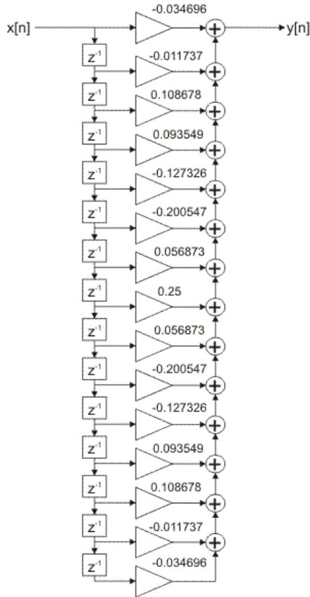
Figure 2-4-5. FIR filter direct realization
