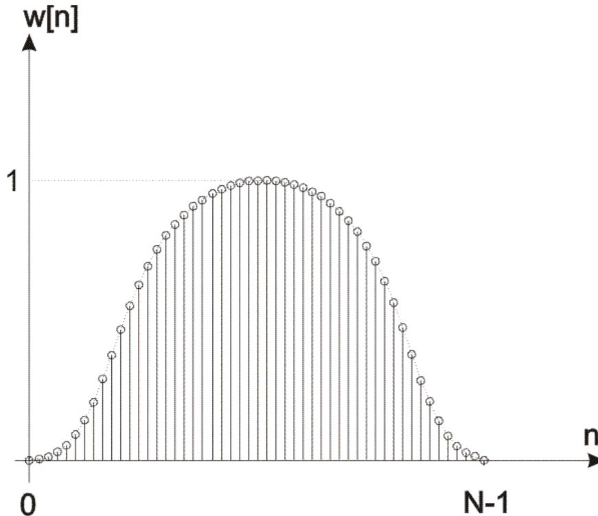
Figure 2-3-6. The Hann window coefficients in the time domain
