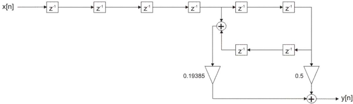
Figure 2-4-53. FIR filter optimized realization structure
