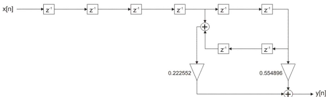
Figure 2-4-61. FIR filter optimized realization structure
