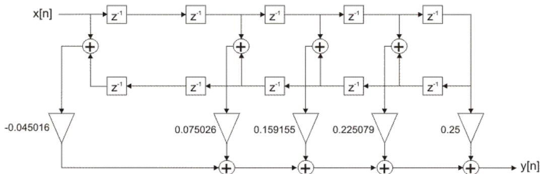
Figure 2-4-2. Optimized realization structure of FIR filter
