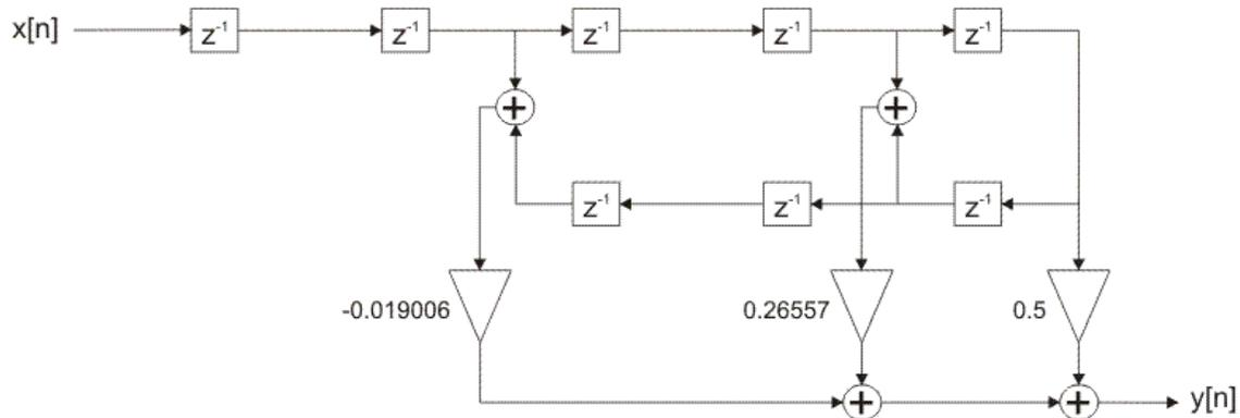
Figure 2-4-44. FIR filter optimized realization structure
