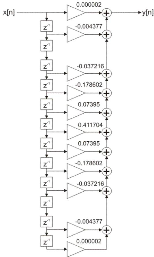
Figure 2-4-66. FIR filter direct realization
