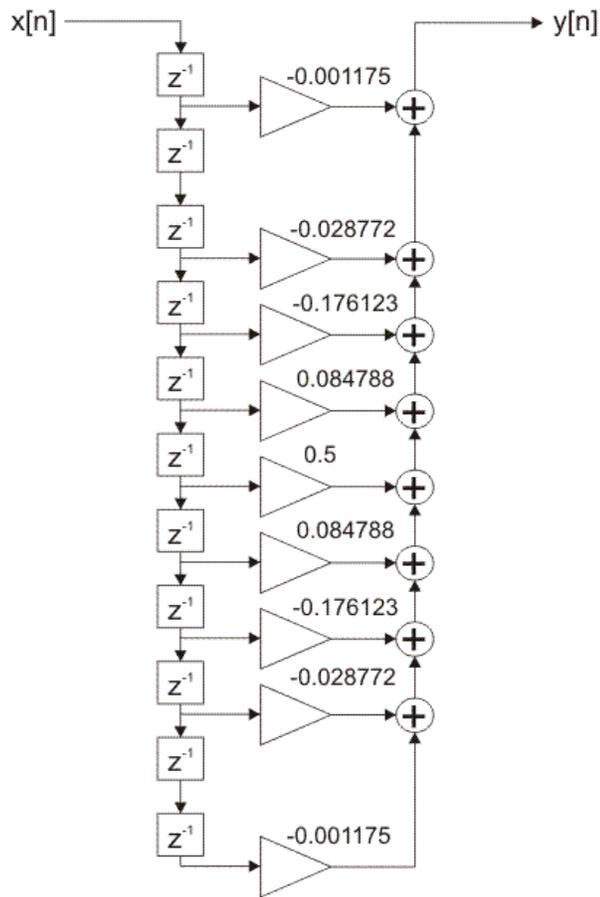
Figure 2-4-50. FIR filter direct realization
