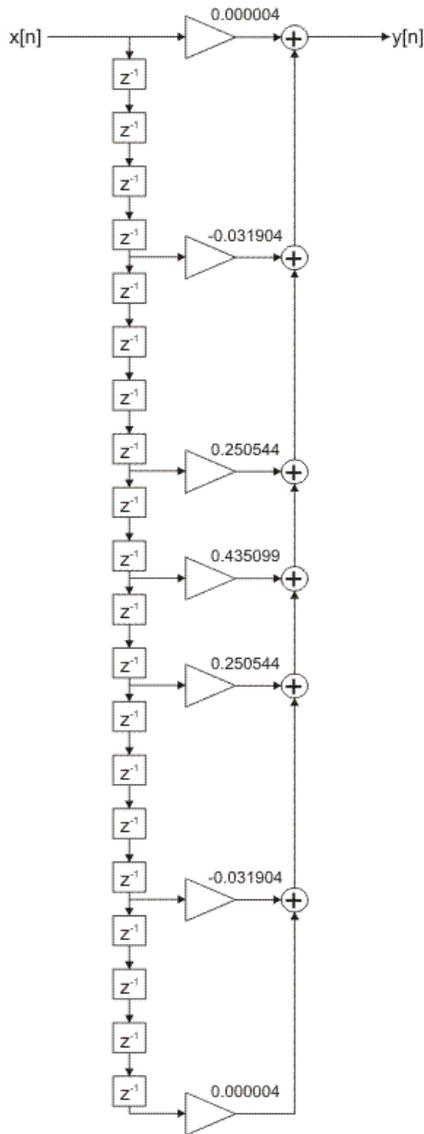
Figure 2-4-68. FIR filter direct realization
