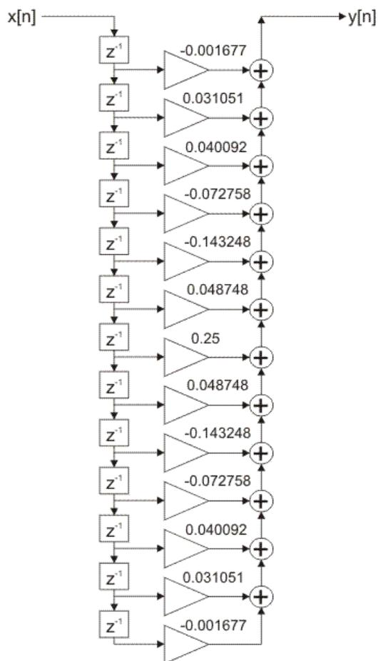
Figure 2-4-13. FIR filter direct realization
