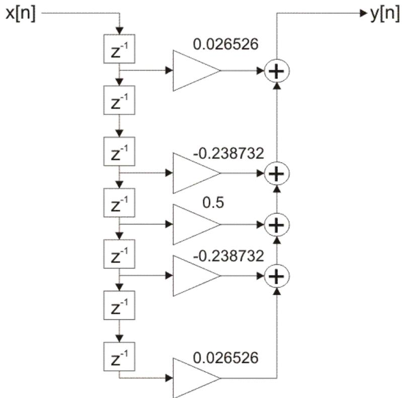
Figure 2-4-11. FIR filter direct realization
