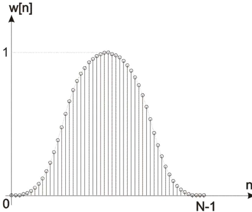
Figure 2-3-14. The Blackman window coefficients in the time domain
