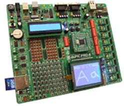
The **dsPICPRO4** supports the latest 64- and 80-pin dsPIC30F microcontrollers from Microchip. It comes with a dsPIC30F6014A. The system includes a USB 2.0 programmer, mikroICD (In-Circuit Debugger), touch panel controller, CAN, RS485, DAC and RTC. [\[more info\]](#)
