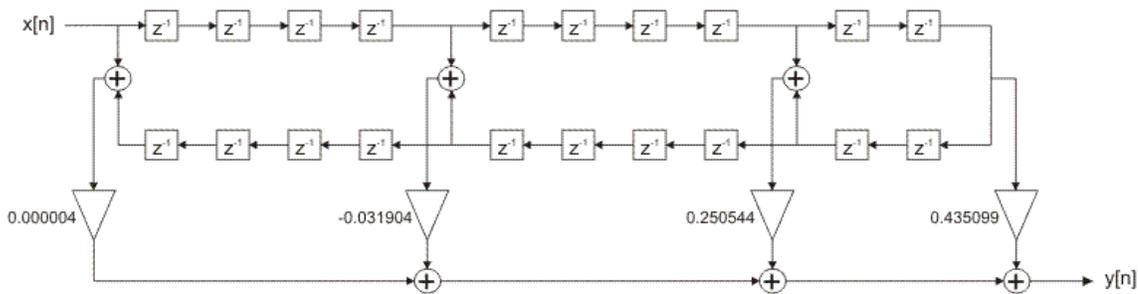
Figure 2-4-69. Optimized FIR filter design
