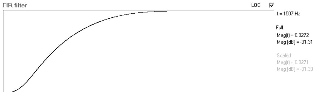
Figure 2-4-46. Frequency characteristic of the resulting filter
