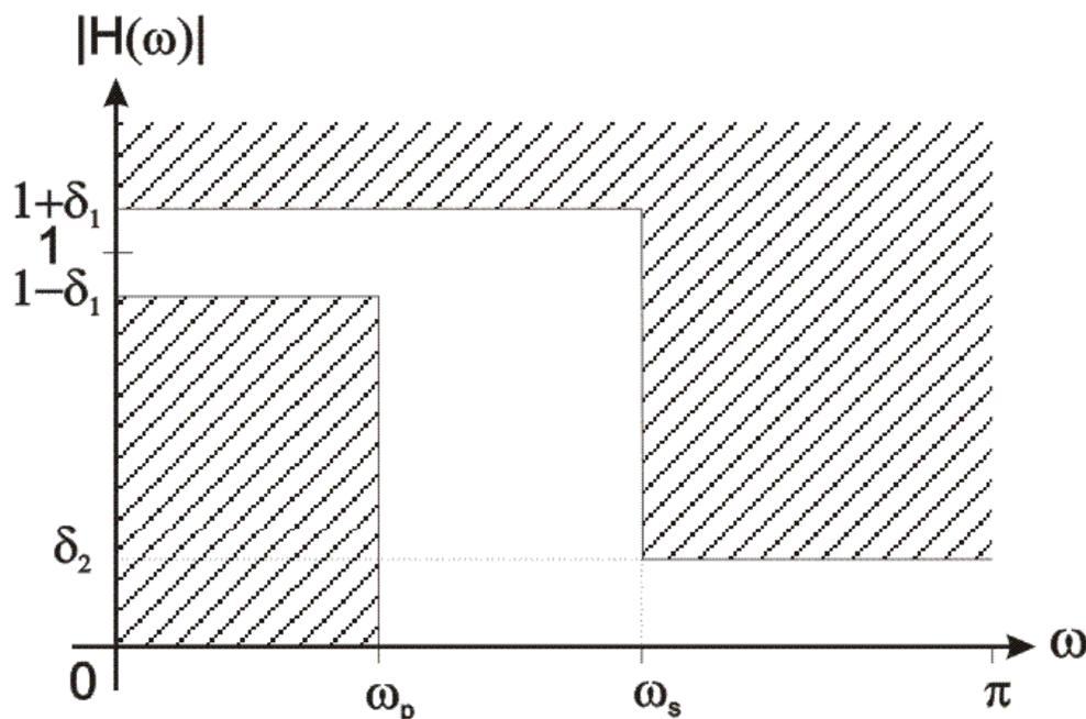
Figure 2-2-1a. Low-pass digital filter specification
