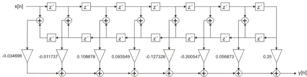
Figure 2-4-6. FIR filter optimized realization structure
