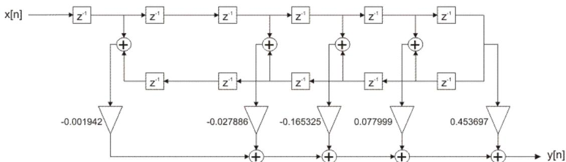
Figure 2-4-59. FIR filter optimized realization structure
