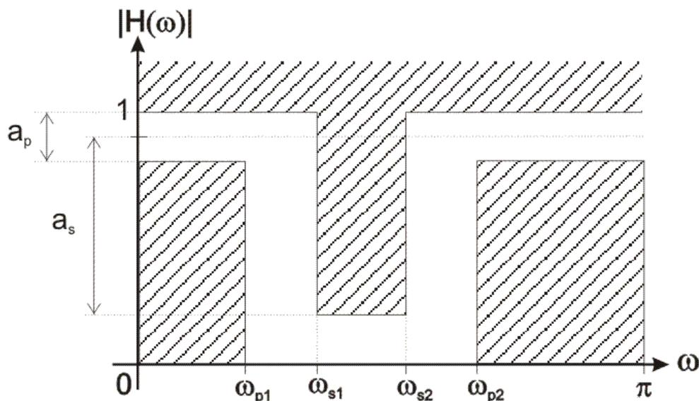
Figure 2-2-4b. Band-stop digital filter specification
