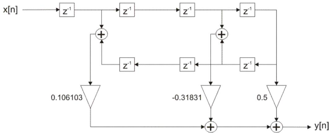
Figure 2-4-4. FIR filter optimized realization structure
