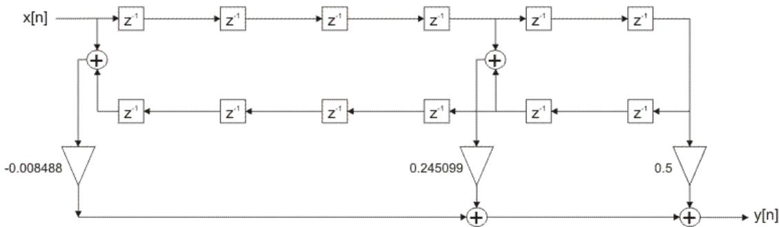
Figure 2-4-42. FIR filter optimized realization structure
