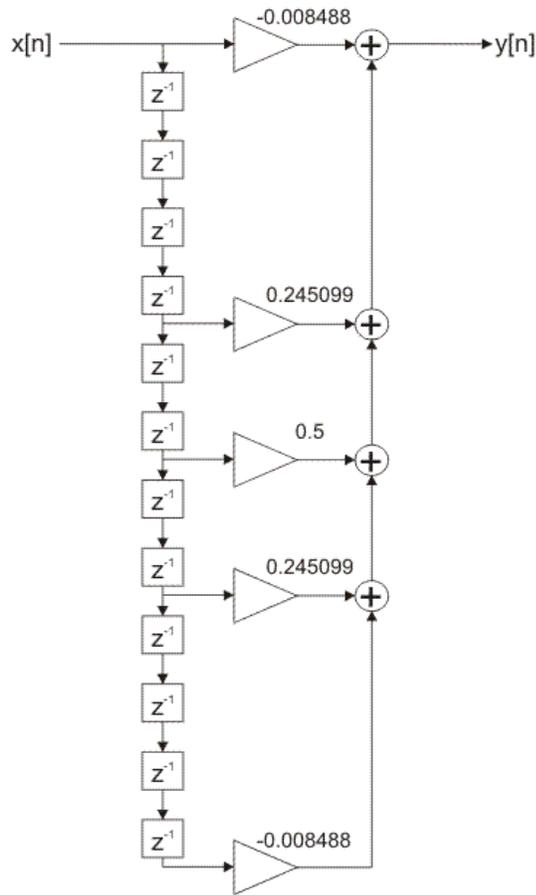
Figure 2-4-41. FIR filter direct realization
