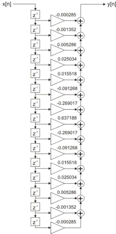
Figure 2-4-48. FIR filter direct realization
