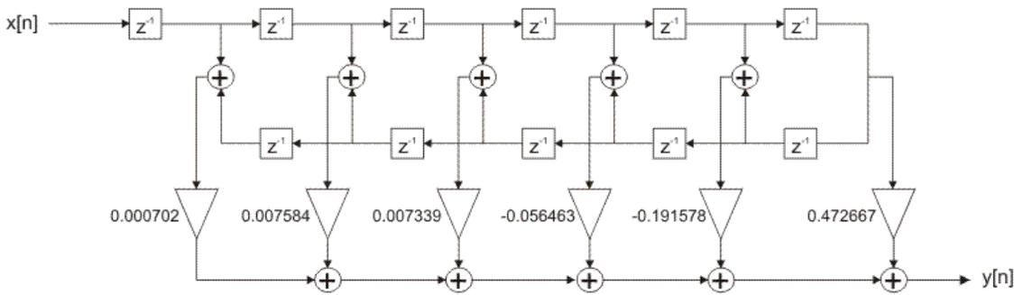
Figure 2-4-57. FIR filter optimized realization structure
