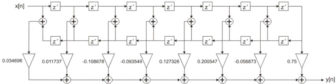
Figure 2-4-8. FIR filter optimized realization structure
