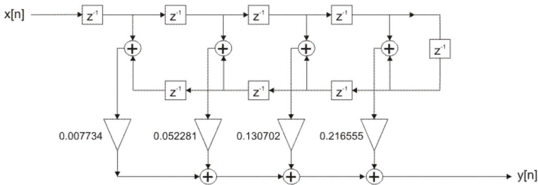
Figure 2-4-10. FIR filter optimized realization structure
