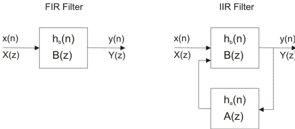
Figure 2-1-1. Block diagrams of FIR and IIR filters
