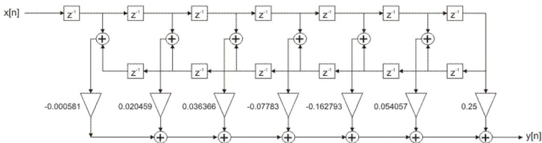
Figure 2-4-22. FIR filter optimized realization structure
