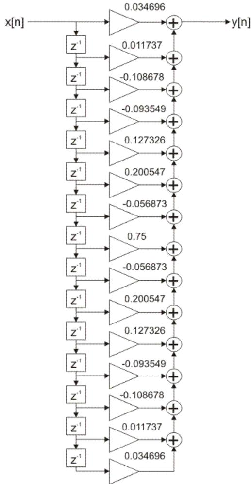
Figure 2-4-7. FIR filter direct realization
