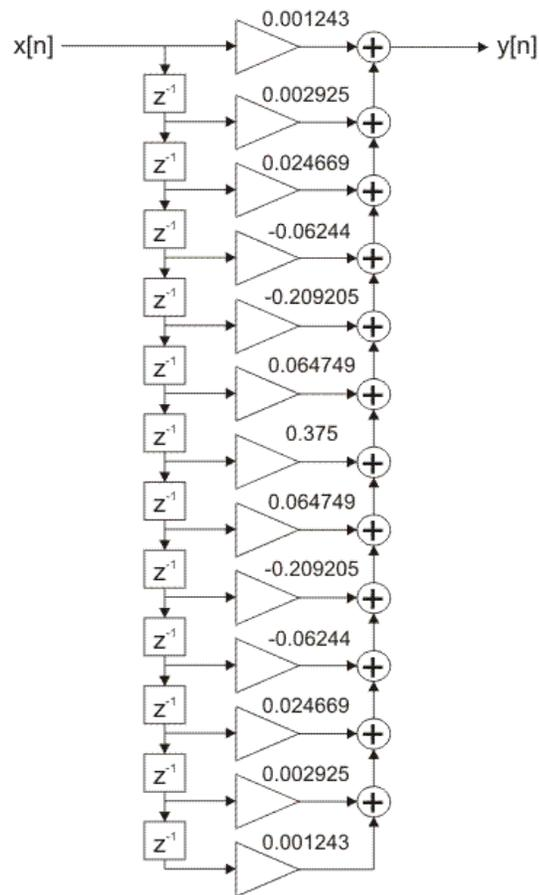
Figure 2-4-39. FIR filter direct realization
