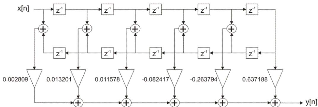
Figure 2-4-38. FIR filter optimized realization structure
