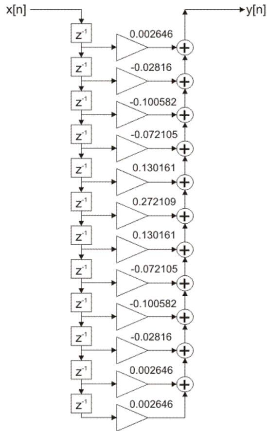
Figure 2-4-29. FIR filter direct realization
