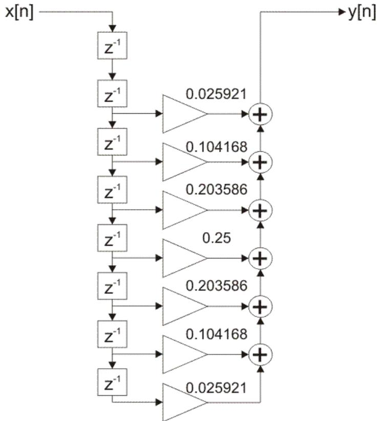
Figure 2-4-17. FIR filter direct realization
