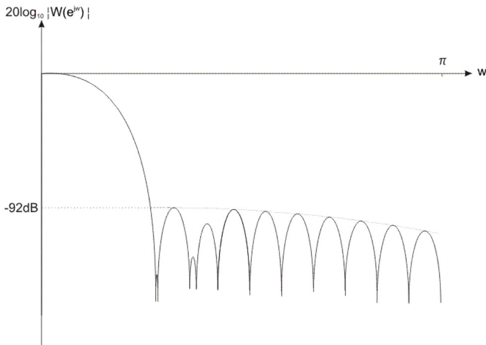
Figure 2-3-17. The Blackman-Harris window coefficients in the frequency domain
