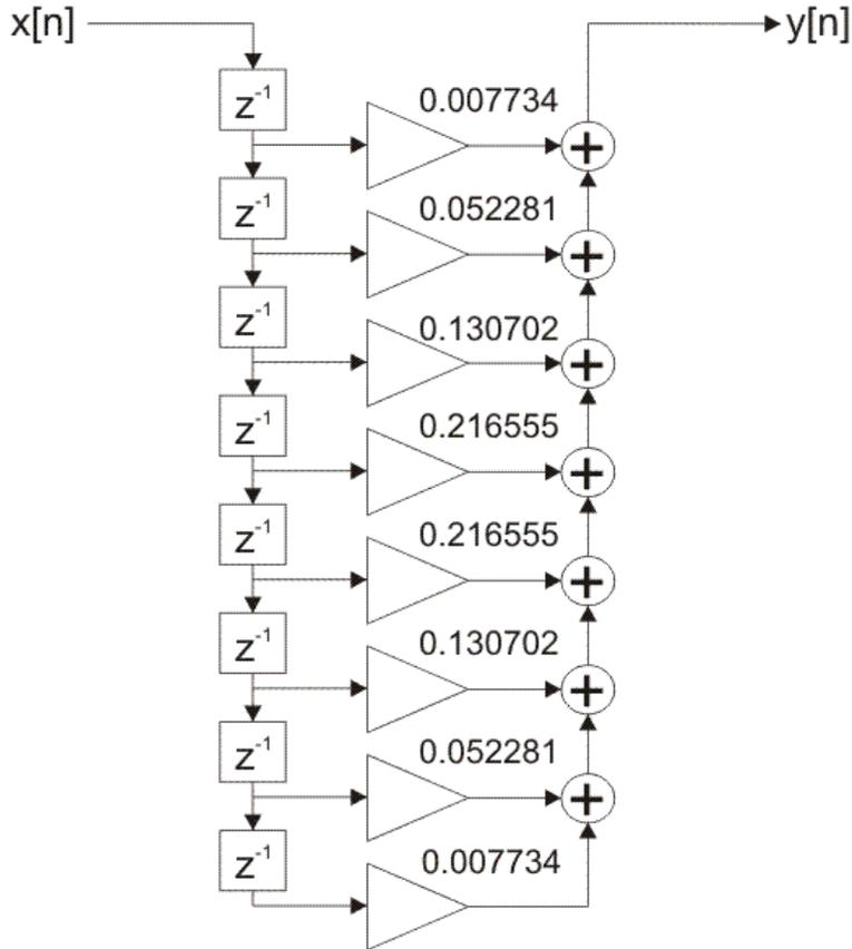
Figure 2-4-9. FIR filter direct realization
