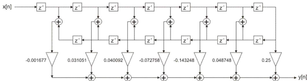
Figure 2-4-14. FIR filter optimized realization structure
