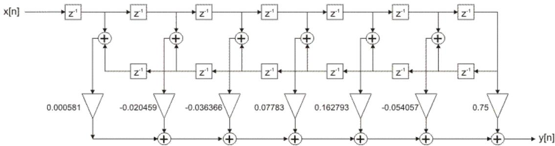
Figure 2-4-24. FIR filter optimized realization structure
