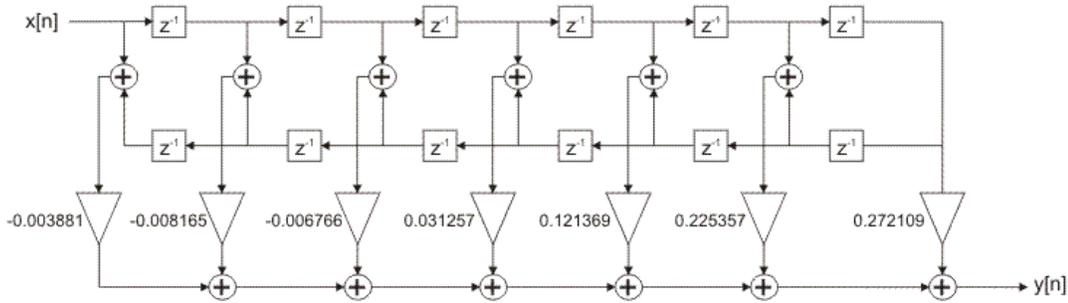
Figure 2-4-36. FIR filter optimized realization structure
