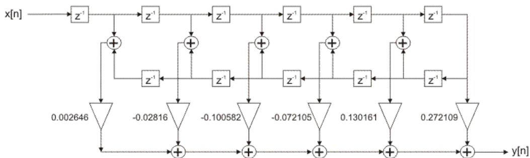
Figure 2-4-30. FIR filter optimized realization structure
