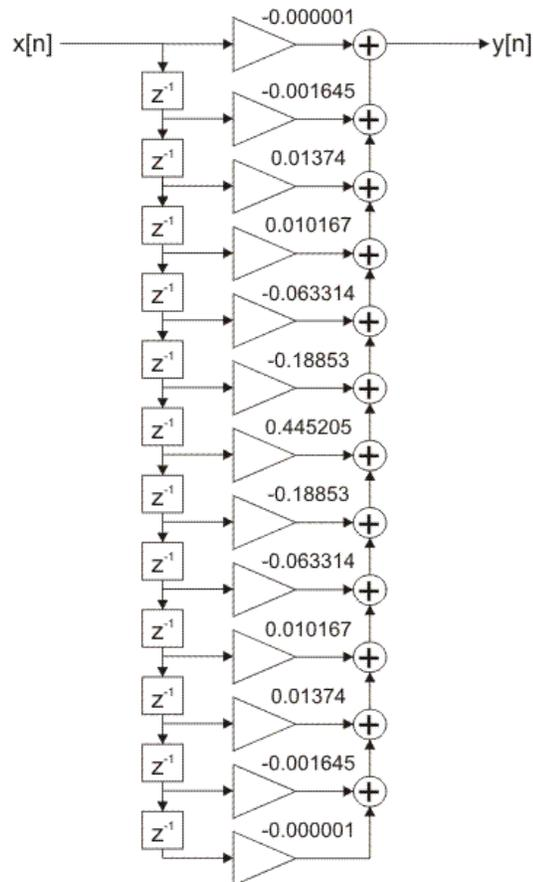
Figure 2-4-64. FIR filter direct realization
