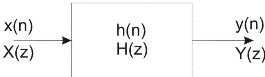
Figure 2-2-7. Block diagram of a linear discrete-time system
