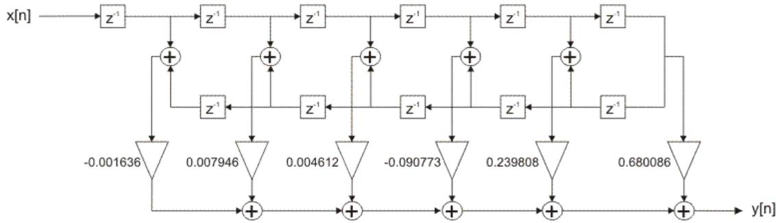
Figure 2-4-55. FIR filter optimized realization structure
