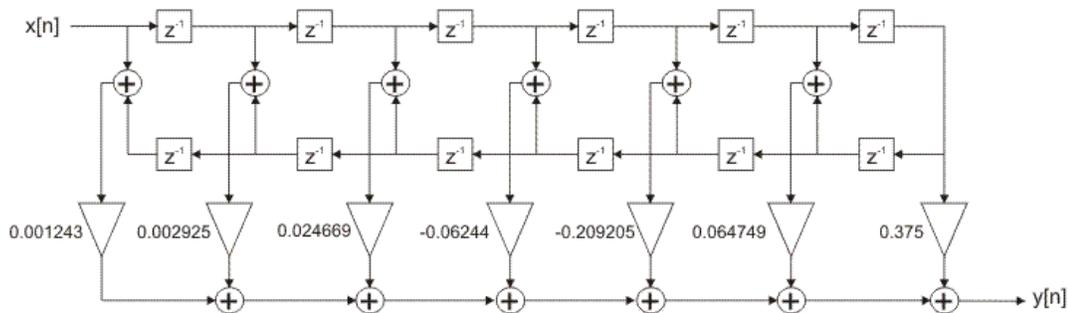
Figure 2-4-40. FIR filter optimized realization structure
