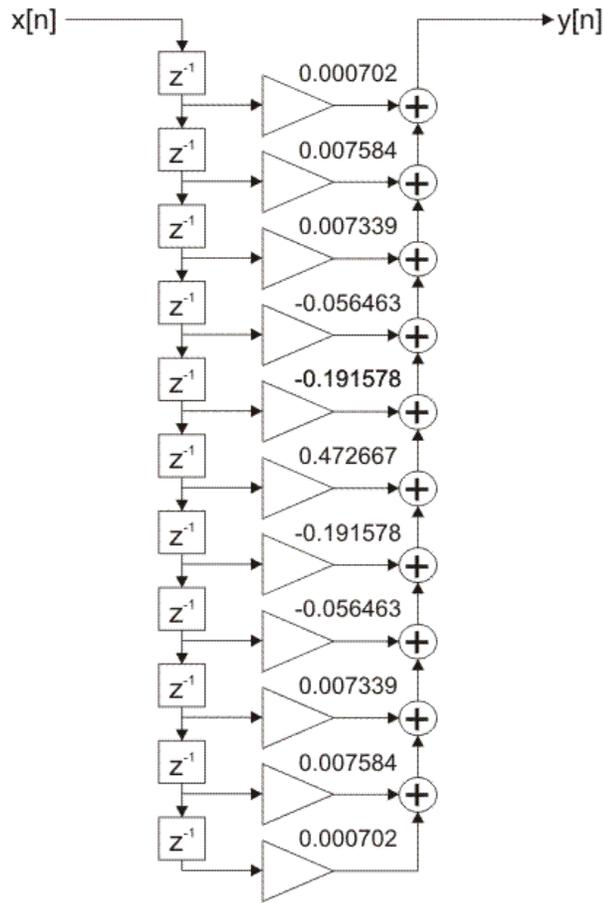
Figure 2-4-56. FIR filter direct realization
