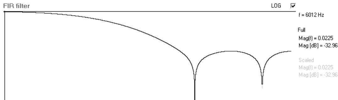
Figure 2-4-33. Frequency characteristic of the resulting filter
