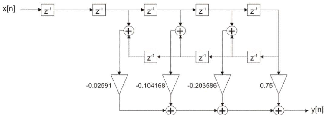
Figure 2-4-20. FIR filter optimized realization structure
