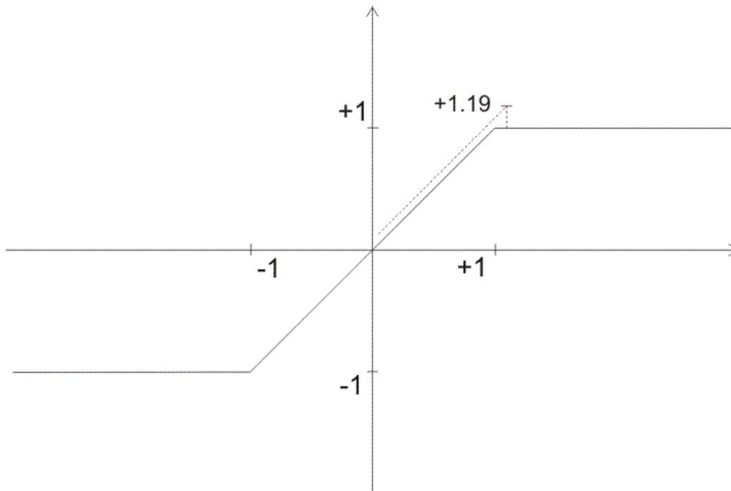
**Figure 2-5-3. Saturation characteristic**
