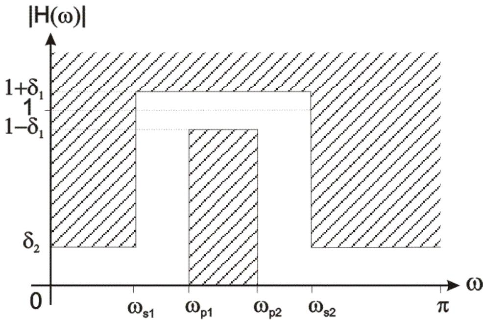
Figure 2-2-3a. Band-pass digital filter specification
