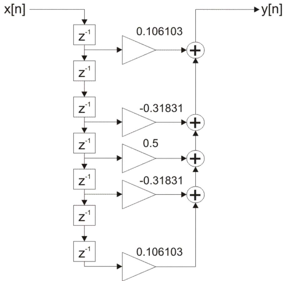
Figure 2-4-3. FIR filter direct realization
