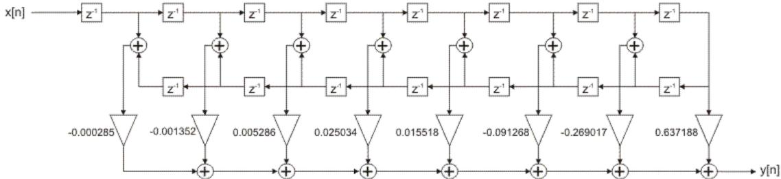
Figure 2-4-49. FIR filter optimized realization structure
