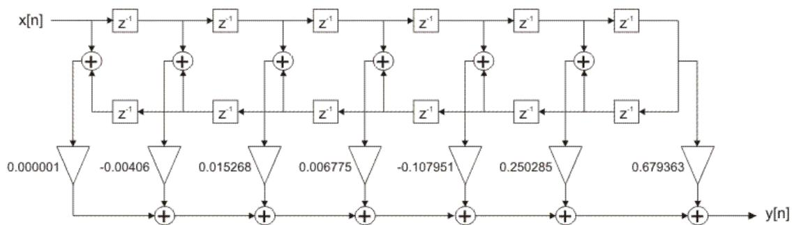
Figure 2-4-63. Optimized FIR filter design
